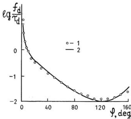
FIG. 1. Aerosol scattering phase function obtained from the observational data (1) and its approximation by a trimodal size distribution function (2).
