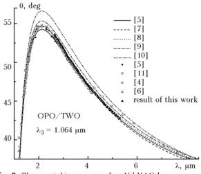
**Fig. 2.** Phase-matching curves for Nd:YAG-laser pumped OPO/TWO of type I. Markers correspond to experimental results.
