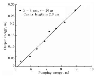
Fig. 3. Output pulse energy of the idler OPO wave as a function of the pump energy.
