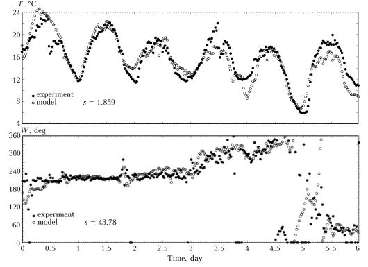
**Fig. 1.** Comparison of the model results with experimental data for air temperature and wind direction at the Aznakaevo station. Time reckoning is from 03:00 of July 1, 2005 with the 30-min interval; *s* is rms deviation of series.
