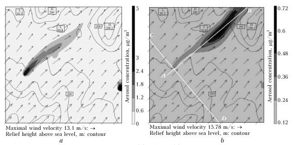
Fig. 3. Aerosol concentration at a height of 30 (a) and 70 m (b) 60 min later the emission beginning.
