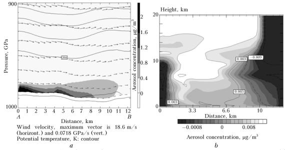
Fig. 4. Vertical slices AB and CD (see Fig. 3) 20 min later the emission beginning: absolute aerosol concentration (a) and the departure from the mean height profile (b).
