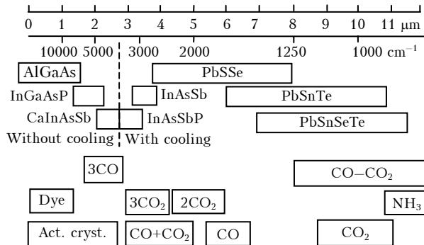
**Fig. 4.** Spectral ranges of radiation wavelengths of different types of lasers (gas, semiconductor, activated crystals, and dye lasers).
