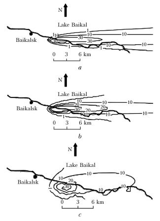
**Fig. 3.** Isolines of calculated values of SO<sub>2</sub> concentrations in the vicinity of BPPP at different values of horizontal component of the coefficient of turbulent diffusion of impurity in the ground layer  $K_x = K_y$ :  $K_x = 50$  (*a*); 100 (*b*); 500 m<sup>2</sup>/s (*c*).
