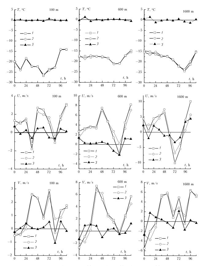
Fig. 2. Temporal behavior of observed measurements (1), retrieved values (2), and current errors (3) in retrieving temperature, zonal and meridional components of wind velocity at individual levels, obtained at the test station Novosibirsk.
