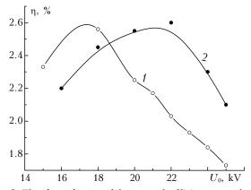
Fig. 3. The dependences of laser total efficiency on charge voltage: for EL-500-100 laser (1); for EL-350-10 laser (2).
