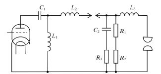
**Fig. 1.** Electric circuit of the laser:  $C_1 = 107$  nF;  $C_2 = 72$  nF;  $L_1 = 100 \mu$ H;  $L_2 = 150$  nH;  $L_3 = 4$  nH;  $R_3$  is current shunt;  $R_1/R_2$  is ohm divider.
