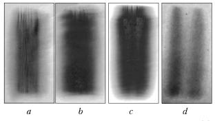
**Fig. 6.** Laser beam patterns: Ne:Xe:HCl = 600:8:1 (*a*); 860:8:1 (*b*); 1000:8:1 at P = 3.8 atm (*c*); Ne:Xe:HCl = = 1800:10:1 at P = 3.6 atm (*d*).
