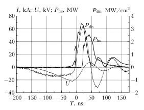
**Fig. 2.** Temporal behavior of voltage U and current I on  $C_2$  capacitor, as well as laser pulse  $P_{\text{las}}$  and specific pumping power  $P_{\text{dis}}$ .
