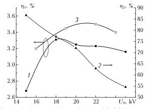
**Fig. 4.** The behavior of laser efficiency: (1), (3) for EL-500-100 and EL-350-10, respectively, and the efficiency of energy transfer from  $C_1$  capacitor to gas discharge plasma (2) depending on the charge voltage for EL-500-100 laser.
