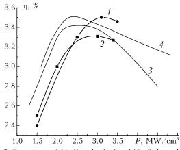
**Fig. 5.** Experimental (1, 2) and calculated (3, 4) dependences of laser operation internal efficiency on specific pump power and halogen concentration in the mixture.
