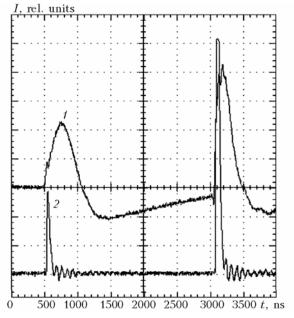
**Fig. 2.** The oscillograms of current (1) and generation (2) pulses at SrII IR-transitions at  $2.6 \,\mu s$  delay between additional and excitation pulses.
