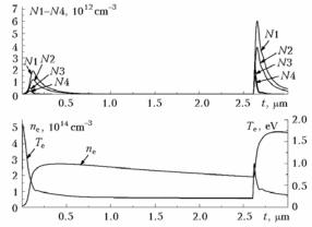
**Fig. 5.** The calculated populations of working levels  $(\lambda = 1.03 \ \mu\text{m}: \text{N4} \rightarrow \text{N2}; \ \lambda = 1.09 \ \mu\text{m}: \text{N3} \rightarrow \text{N1})$ , concentration  $n_{\text{e}}$  and electron temperature  $T_{\text{e}}$ .
