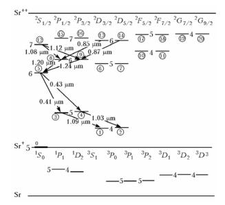
Fig. 3. The scheme of levels of strontium atom and ion (the arrows indicate SrII transitions, at which laser generation is observed, the numbering of SrII levels used in mathematical model is shown in circles).
