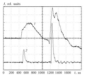
Fig. 1. The oscillograms of current (1) and generation (2) pulses at SrII IR-transitions at 0.72  $\mu$ s delay between additional and excitation pulses.
