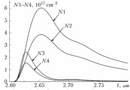
Fig. 6. The calculated populations of working levels ( $\lambda = 1.03 \ \mu m$ : N4  $\rightarrow$  N2;  $\lambda = 1.09 \ \mu m$ : N3  $\rightarrow$  N1) in the second excitation pulse.
