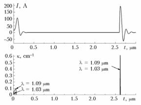
**Fig. 4.** The calculated additional and excitation current pulses and amplification coefficients at SrII IR-transitions at a 2.6 µs delay.
