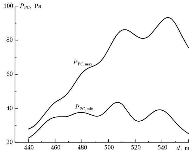
**Fig. 3.** Amplitude-spatial distribution of the acoustic pressure fields formed along the beam propagation path.
