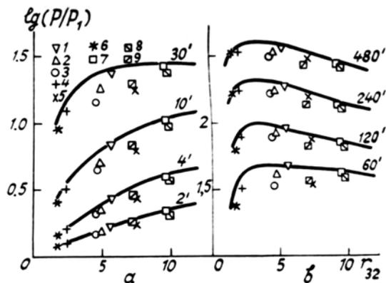
FIG. 2. Dependence of MS input to lidar returns on the integral parameters  $r_{32}$  of the size spectra.
