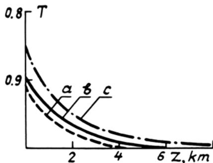
FIG. 4. Transmittance of a vertical atmospheric path from ground level to height  $z$  for radiation of various types of PL's.
