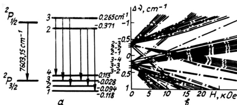
FIG. 1. Hyperfine structure of iodine photodissociation laser transitions (a — in the absence of a magnetic field; b — Zeeman splitting in a constant magnetic field up to 30 kOe)
