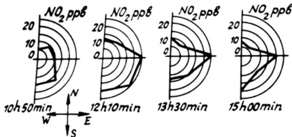
FIG. 3. The result of measurements of the nitrogen dioxide concentration as a function of the azimuthal angle in the town of Dolgoprudnyi on March 23, 1989
