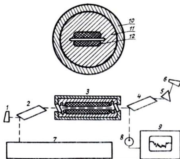
FIG. 1. Flow-chart of the experimental set-up: resonator cavity mirrors (1, 6), active elements (2, 4), high-pressure cell with capacitor plates 12 (3), prism (5), spectrograph (7), photodetector (8), oscillograph (9), steel case (10), isolator (11).
