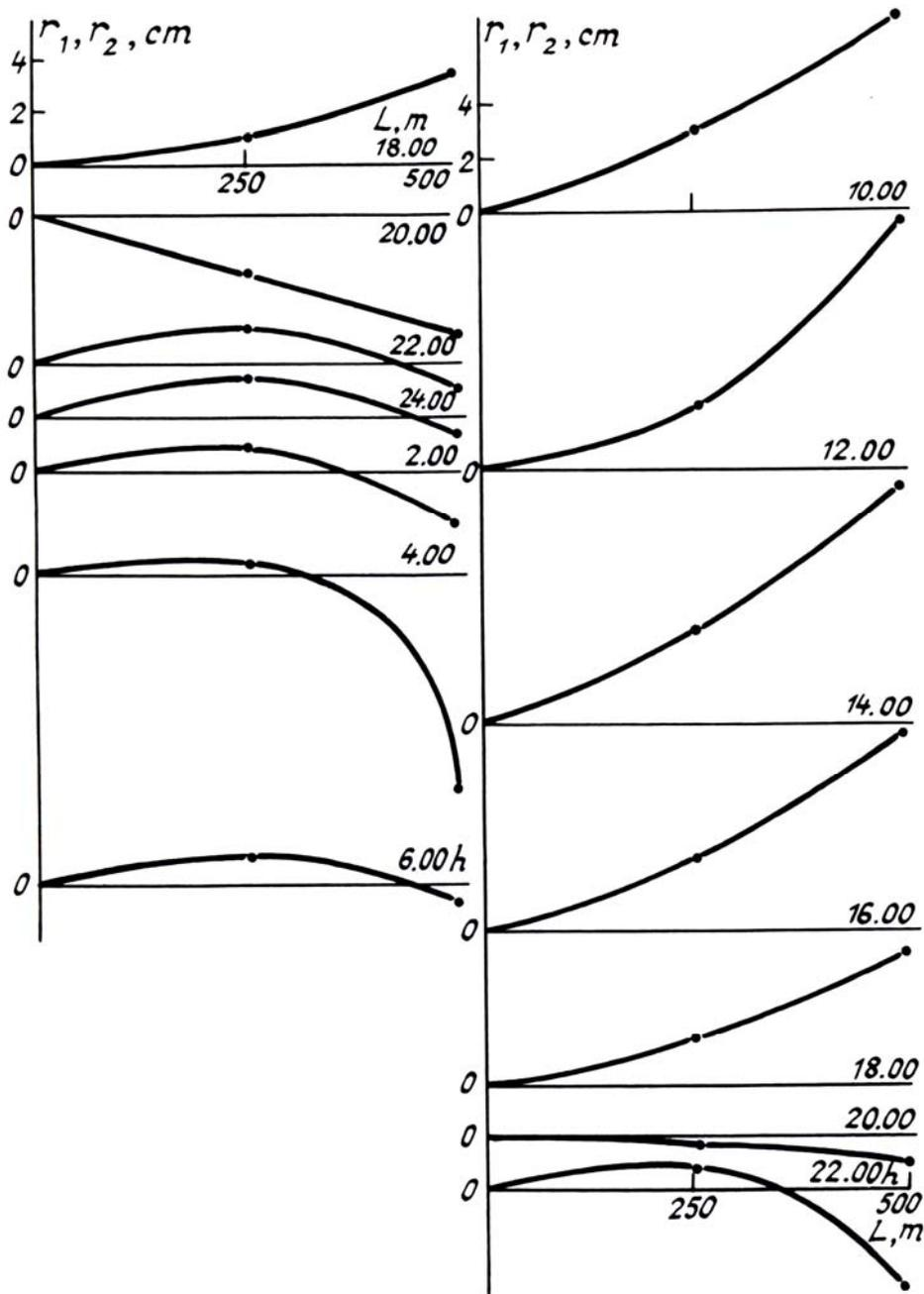
FIG. 2. Temporal trends of refract distortions at distances of 250 and 500 m.
