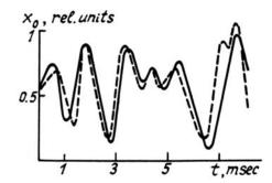
FIG. 2. Measurements of the amplitude of the oscillations. The solid line shows the measurements performed with a Doppler autodyne and the dashed line shows the measurements performed with a piezoelectric transducer.
