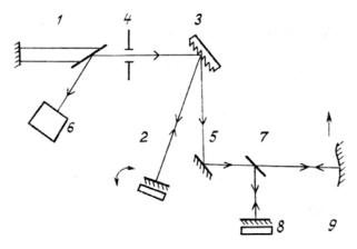
FIG. 5. Block diagram of autodyne with frequencytunable laser: 1) gas-discharge tube of CO<sub>2</sub> laser: 2) cavity mirror mounted on a piezoelectric corrector; 3) diffraction grating; 4) diaphragm; 5) rotating mirror; 6) photodetector; 7) beamsplitter; 8) mirror on piezoelectric corrector; 9) reflecting surface.
