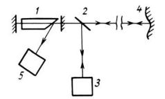
FIG. 4. Block diagram of autodyne with a frequency shift: 1)  $CO_2$  laser; 2) beam-splitter; 3) frequency shifter; 4) surface; 5) photodetector.
