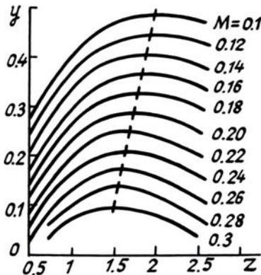
FIG. 2. The function  $y$  given by Eq. (14) versus the normalized interval of observation  $z$  for different values of the parameters  $M$  for signal-to-noise ratio  $q^2 \geq 100$ .
