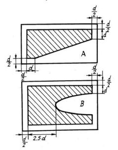
FIG. 3. Electrode shapes for LiNbO<sub>3</sub> samples, d is the crystal thickness
