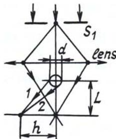
FIG. 2. Light diffraction by a wire.
