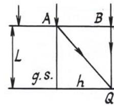
FIG. 4. Diffraction of a plane wave by a screen with a straight edge.
