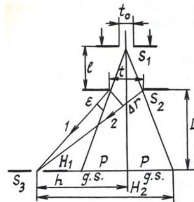
FIG. 1. Block diagram of a cylindrical wave incident on the slit.
