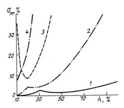
FIG. 4. The absolute error in measuring the relative humidity at a height of 100 m in the presence of wind with a velocity of 5 m  $\cdot$  s<sup>-1</sup>.
