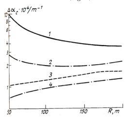
FIG. 1. The turbulent shift in the difference of the sound absorption coefficients under almost calm conditions.
