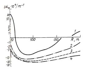
FIG. 2. The turbulence-wind shift in the difference of the sound absorption coefficients with a wind velocity of 5 m  $\cdot$  s<sup>-1</sup>.
