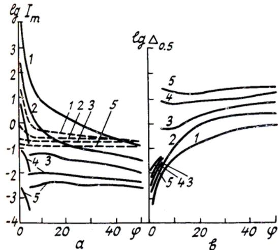
FIG. 2. The amplitude  $I_m$  (a) and the pulse width  $\Delta_{0.5}$  (b) versus the angle of observation  $\varphi$ .
