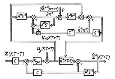
FIG. 1. Block diagram of the adaptive filter.
