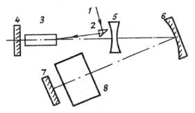
FIG. 1. Optical diagram of the laser. 1) pump radiation, 2) rotating prism, 3) active element, 4) output mirror, 5) negative lens, 6) spherical mirror, 7) nontransmitting mirror, and 8) selector.
