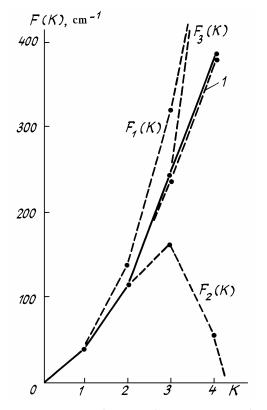
FIG. 1. Experimental (solid line) and calculated (dashed lines) values of the ground-state rotational energy (the component V = 1) of the (HF)<sub>2</sub> dimer (for the hypothetical level J = 0). Dashed lines correspond to the results of calculation with the polynomial representation of  $F_N(K)$ incorporating the N adjustable parameters determined by fitting the N experimental data. Curve 1 corresponds to the results of calculation with two-parametric function (11).
