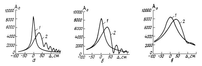
FIG. 2. Dependence of amplitude  $A_0$  on the value  $\Delta$  (1) PA and 2) exact solution) at different values of the geometrical divergence  $\alpha = a/f$ :  $\alpha = 2/30$  (a), 2/45 (b), and 2 cm/70 cm (c). The boundary beam is of Gaussian type and m = 1.5.
