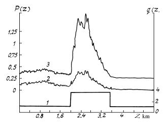
FIG. 1. Correction of the lidar signal with an account of the function  $q_{ik}$ : 1) correcting function g(z) retrieved from the lidar return by Eqs. (8)–(10), 2) corrected lidar return, and 3) initial lidar return signal; curves 2 and 3 are shifted one and two scale divisions upward, respectively.
