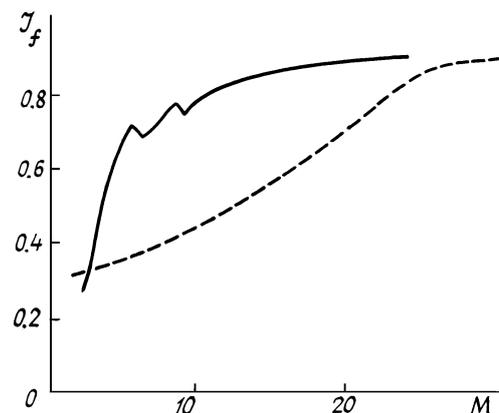
FIG. 2. Criterion of focusing  $J_f$  vs the number of its measurements  $M$  in the process of optimization. Solid line denote the simplex method, dashed line – gradient method. Path is of length  $z_0 = 0.5$  and the parameter of nonlinearity  $R_V = -28$ .
