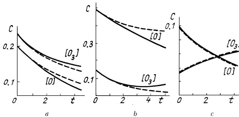
FIG. 5. Variants of time behavior of concentrations for systems in the (y, z) plane with constant dashed curve) and arbitrary (solid curve) concentration of O<sub>2</sub> for A = 1. a, b) x<sub>0</sub><sup>2</sup> = 0,0025 and c) x<sub>0</sub><sup>2</sup> = 0,16.
