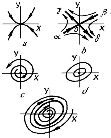
FIG. 7. Types of steady states: a) stable node, b) saddle, c) unstable focus, d) center, and e) stable limit cycle.
