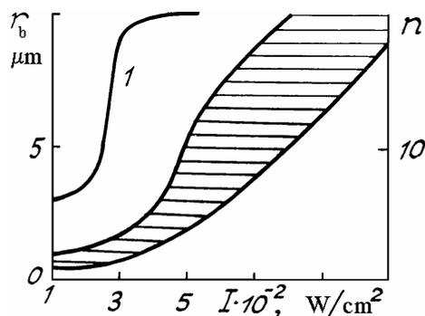
FIG. 2. The effect of the energy contribution of the ILR on the radius of the bubble (curve 1) located in the region of the main maximum of heat release and on the total number of bubbles in the volume of the quartz particle with radius  $a_0 = 70 \mu\text{m}$  (hatched area).
