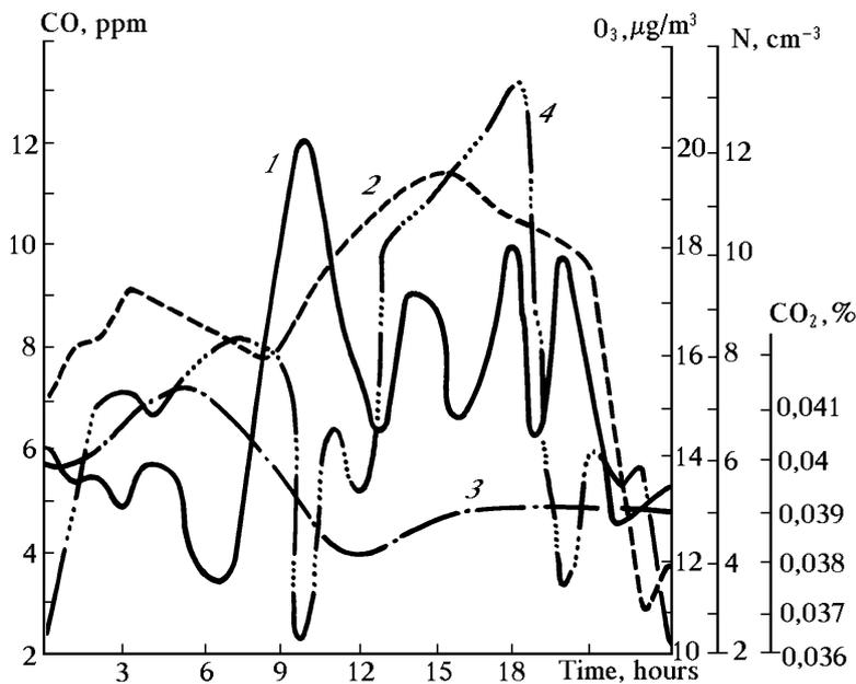
FIG. 6. The diurnal behavior of aerosol, carbon oxide, carbon dioxide, and ozone in fall. Designations are the same as in Fig. 5.
