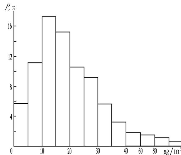
FIG. 2. Recurrence of different values of ozone concentration in the ground air layer.
