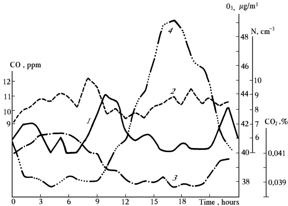
FIG. 5. The diurnal behavior of the number densities: 1) aerosol, 2) carbon oxide, 3) carbon dioxide, and 4) ozone in summer.
