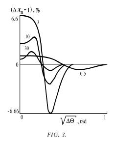
Depicted in Fig. 3 are the normalized dependences of the PSF width on the angle between the direction of illumination and observation calculated from the formula
