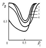
FIG. 3. The SEO detection probability as a function of the coefficient of the object interelement correlation  $\rho_1$  for object dimensions 7×7 (curves 2, 3) and 5×5 (1, 4); the ratio of the variances of the intensity of the object and background images is  $\varepsilon^2 = 1$  (1, 3), 0.8 (2), and 0.5 (4); the background interelement correlation coefficient is  $\rho_0 = 0.5$
