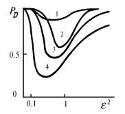
FIG 4. The SEO detection probability as a function of the ratio of the variances of the intensities of the object and background images  $\varepsilon^2$  for different values of the interelement correlation coefficients  $\rho = \rho_0 = \rho_1 = 0.7$  (1) and 0.5 (2–4) and the object
