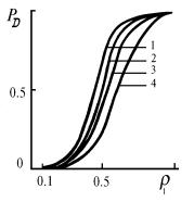
FIG. 2. The SEO detection probability as a function of the interelement correlation coefficient  $\rho = \rho_0 = \rho_1$  for equal variances of the intensities of the object and background images ( $\epsilon^2 = 1$ ) and different object dimensions: 1) 10×10; 2) 12×2; 3) 5×5; and, 4) 3×3.
