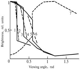
FIG. 3. Normalized brightness distribution over the input pupil of the OES.  $z_{st} = 0.01 \text{ m}$ : 1) h = 100 m,  $\sigma^2 = 0$ ; 2) h = 100 m,  $\sigma^2 = 0.2$ ; 3) h = 50 m,  $\sigma^2 = 0$ ; 4) h = 50 m,  $\sigma^2 = 0.2$ ; 5) h = 30 m,  $\sigma^2 = 0$ ; 6) h = 30 m,  $\sigma^2 = 0.2$ , and  $z_{st} = 0.51 \text{ m}$ , and 7) h = 30 m,  $\sigma^2 = 0$ .
