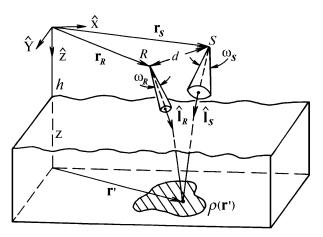
FIG. 1. Generalized scheme of the opto-electronic system of observation.
