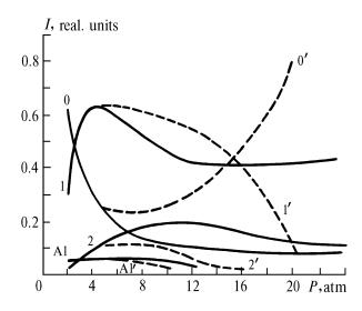
FIG. 4. Dependence of the intensity of components of the SRS conversion on the pressure: in pure hydrogen (A1, 0, 1, and 2), in hydrogen under initial pressure of 4 atm with subsequent addition of argon (A1', 0', 1', and 2').  $\lambda = 532$  (0), 683 (1), 954 (2), and 436 (A1) nm.
