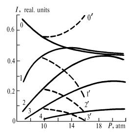
FIG. 2. Dependence of the intensity of components of the SRS conversion on the pressure: in pure hydrogen (0, 1, 2, 3, and 4); in hydrogen under initial pressure of 10 atm (0', 1', 2', and 3') with subsequent addition of argon.  $\lambda = 308 (0), 353 (1), 413 (2), 499 (3), and 628 nm (4).$
