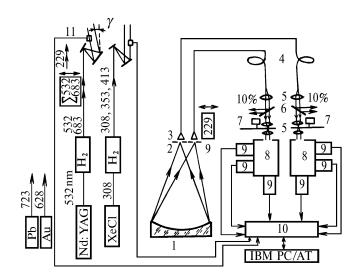
FIG. 1. Block diagram of the lidar. Receiving mirror (1), field diaphragms (2), focons (3), light guides (4), lenses (5), light-splitting mirrors (6), mechanical shutter (7), cells of spectral selection (8), PMT (9), photon counter (10), and phototransistors (11).
