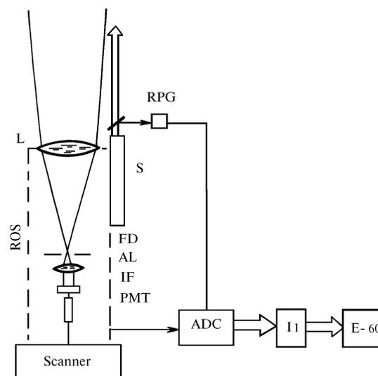
FIG. 1. Configuration of the LISA lidar.
