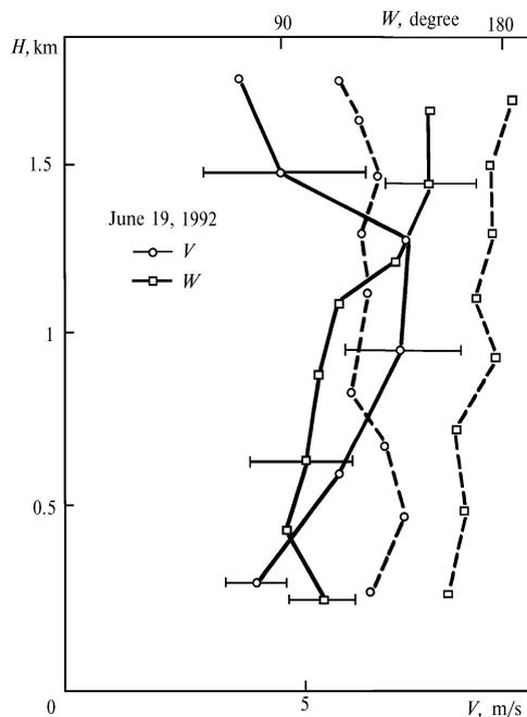
FIG. 2. Profiles of the wind speed  $V$  and direction  $W$  measured by the lidar and METEOR station on June 19, 1991. Horizontal bars indicate the 0.9 confidence level.
