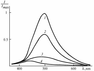
FIG. 2. Fluorescence spectra of the compound II in ethanol as a function of concentration of the sulfuric acid admixture: C = 0 (1), 0.01 (2), 0.03 (3), and 0.05 mole/liter (4).
