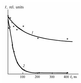
FIG. 4. Kinetics of intensity variation of the  $S_1 - S_n$ absorption intensity for different wavelengths of the probing radiation  $\lambda = 740$  nm (1) and  $\lambda = 547$  nm (2).
