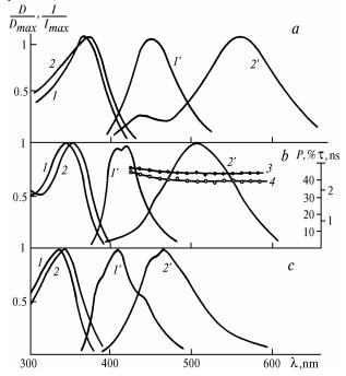
FIG. 1. Absorption spectra (1, 2), fluorescence spectra (1', 2'), polarization spectra of fluorescence (3), and spectral dependence of the fluorescence duration (4) of the compounds I(a), II(b) and III(c) in toluene (1, 1') and ethanol (2, 2'). D is the optical density and I is the fluorescence intensity in rel. units.
