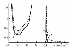
FIG. 1. Absorption spectra for solution of coumarin 2. 1) before and 2) after generation, 3) solution after regeneration.
