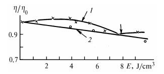
FIG. 4. C2 decay curves in monopulse (2) and repetition (5 Hz) modes (1). Arrow points the start regeneration in repetition mode.
