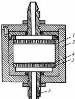
FIG. 3. Regeneration fitter for the active medium.
