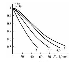
FIG. 2. Relative efficiency  $(\eta/\eta_0)$  of C2 generation vs energy pumped per unit volume of solution: 1) pure ethanol solution;
