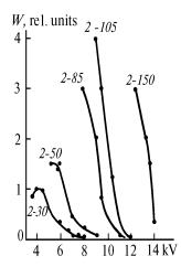
FIG. 3. Dependence of the losing power at the  $1.45-\mu m$ neon line on voltage for the third-type device. The first number means the neon pressure and the second (after dash) – the helium pressure, capacitance is  $0.4 \mu F$ .
