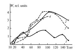
FIG. 4. Dependence of the maximum lasing power at the 1.45- $\mu$ m neon line on the helium pressure for the third type device. The neon pressure is 1 (1), 2 (2), 4 (3), and 8 Torr (4), and capacitance is 0.4  $\mu$ F.
