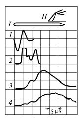
FIG. 2. Dynamics of the processes developing in the chamber of the first-type device. I is a photoscan schematic in tube and II is a photoscan schematic in the chamber. 1) Current, 2) losing at the 2.026  $\mu$ m neutral xenon line in chamber, 3) spontaneous emission in chamber (588.9 nm neutral helium line), and 4) 840 nm neutral xenon line. Helium pressure is 150 Torr. Xenon pressure is 1 Torr, capacitance is 0.4  $\mu$ F, and voltage is 14 kV.
