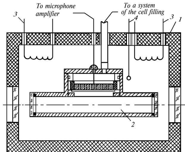
FIG. 1. Block diagram of the thermal PA cell: 1) thermostat, 2) PA cell, 3) heating elements, and 4) thermocouple.
