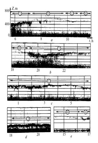
FIG. 1. The sodar recording of elevated inversions of various intensity. a - January 19, 1991 (morning); b - March 20, 1991; c - January 21, 1991; d - November 26, 1991; and, e - January 19, 1991 (day).
