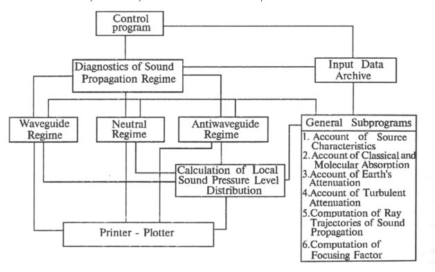
FIG. 1. Flowchart of the software package AOS (Acoustics of Open Space).
