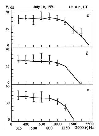
FIG. 3. Sound pressure level, in dB, in the case of waveguide regime for different path lengths as a function of the frequency f of radiated signal, d = 3000 (a), 4500 (b), and 6000 m (c). Solid curves are for the calculated results; circles are for the measured values. Vertical bars denote the confidence intervals.
