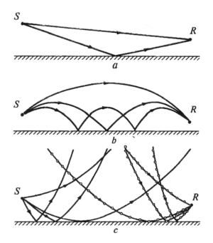
FIG. 2. Ray patterns for acoustic noise propagation in the atmosphere under various meteorological conditions: a) neutral regime; b) waveguide regime (only the topbottom rays are shown); and, c) antiwaveguide regime. Here S is the noise source, R is the receiver (observation point), ----- – direct rays,  $\circ-\circ-\circ-$  – the scattered rays.
