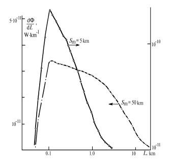
FIG. 3. Differential fluxes of backscattered radiation. Opto-geometrical parameters of lidar visibility meter:  $P_0 = 4.5 \cdot 10^{-2} \text{ W}, \quad 2\gamma_{\rm s} = 5', \quad d_{\rm s} = 0.005 \text{ m}, \quad 2\gamma_{\rm r} = 22', \quad d_{\rm r} = 0.1 \text{ m}, \quad B = 0.2 \text{ m}, \quad \varphi = 0^{\circ}.$
