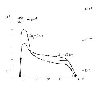
FIG. 4. Differential fluxes of backscattered radiation. Opto-geometrical parameters of lidar visibility meter:  $P_0 = 4.5 \cdot 10^{-2} \text{ W}, \quad 2\gamma_s = 5', \quad d_s = 0.005 \text{ m}, \quad 2\gamma_r = 1^\circ,$  $d_r = 0.16 \text{ m}, B = 0.25 \text{ m}, \varphi = 55'.$
