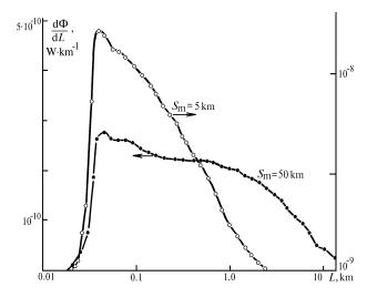
FIG. 2. Differential fluxes of backscattered radiation. Opto-geometrical parameters of lidar visibility meter:  $P_0 = 4.5 \cdot 10^{-2} \text{ W}, \quad 2\gamma_s = 5', \quad d_s = 0.005 \text{ m}; \quad 2\gamma_r = 1^\circ;$  $d_r = 0.1 \text{ m}, B = 0.2 \text{ m}; \varphi = 0^\circ.$
