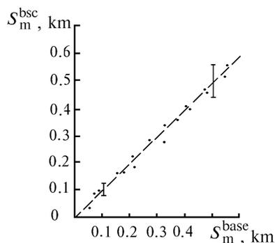
FIG. 3. Results of simultaneous measurements of  $S_m$  by the backscatter ( $y$ -axis) and base ( $x$ -axis) MVR meters.
