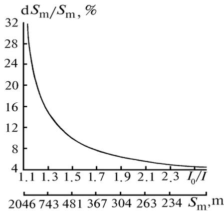
FIG. 2. Relative rms error in measuring  $S_m$  by the base method. The scale of  $S_m$  is shown for  $L = 50$  m.
