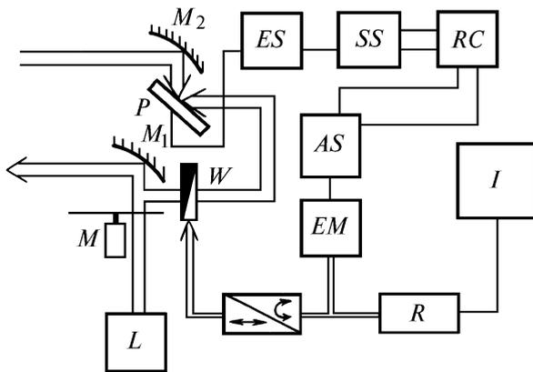
FIG. 1. Functional diagram of the backscatter meteorological visibility range meter, where ES is the electronic system, SS is the synchro switch, and RC is the reversible counter.
