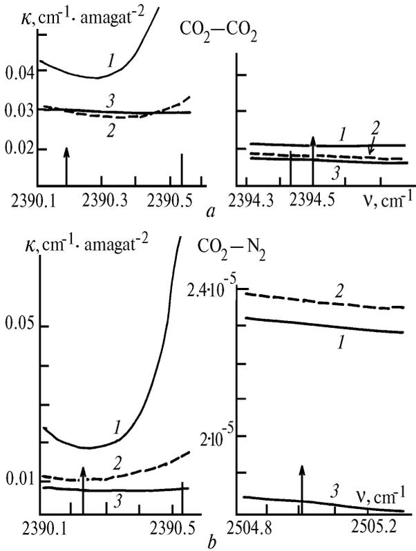
FIG. 3. Change in the character of the temperature dependence of the  $\text{CO}_2\text{-CO}_2$  (a) and  $\text{CO}_2\text{-N}_2$  (b) absorption coefficients in the vicinity of several sensing channels (marked by arrows). The curves correspond to temperatures of 300 (1), 250 (2), and 190 K (3).
