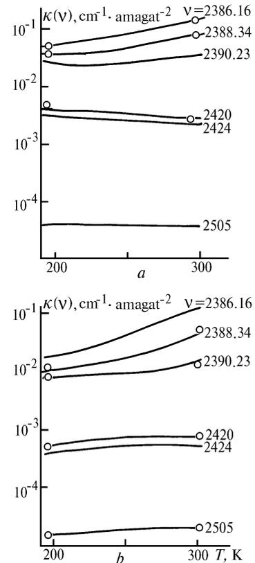
FIG. 2. Temperature dependence of the  $\text{CO}_2$ - $\text{CO}_2$  (a) and  $\text{CO}_2$ - $\text{N}_2$  (b) absorption coefficients in the 4.3  $\mu\text{m}$  band at several frequencies given to the right of the curves.
