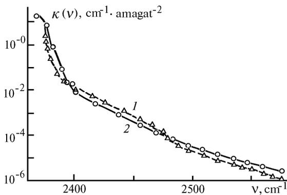
FIG. 1. The  $\text{CO}_2$  absorption coefficient in the 4.3  $\mu\text{m}$  band wing at  $T = 193$  K (curve 1) and at  $T = 296$  K (curve 2) calculated on the basis of the line wing theory. Experimental data are taken from Ref. 6:  $\circ$  – 296 K and  $\Delta$  – 193 K.
