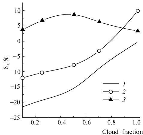
FIG. 7. Values of  $\delta$  for  $\xi_{\infty} = 0^\circ$ ,  $\sigma = 30 \text{ km}^{-1}$ , and  $D = H = 0.5 \text{ km}$ : stratus (1) and "Lambertian" clouds (2 and 3); the underlying surface albedo  $A_s = 0$  (1 and 2) and  $A_s = 0.8$  (3).
