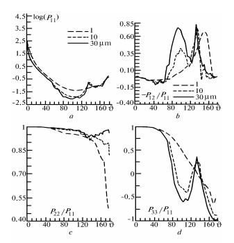
FIG. 1. Angular dependences of reduced values of the light scattering phase matrix elements for ensembles of circular cylinders uniformly oriented in horizontal plane with different mean geometric radii.
