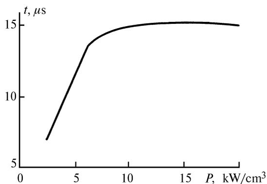
FIG. 4. Amplification pulse duration in the XeCl medium as a function of the specific pumping power.
