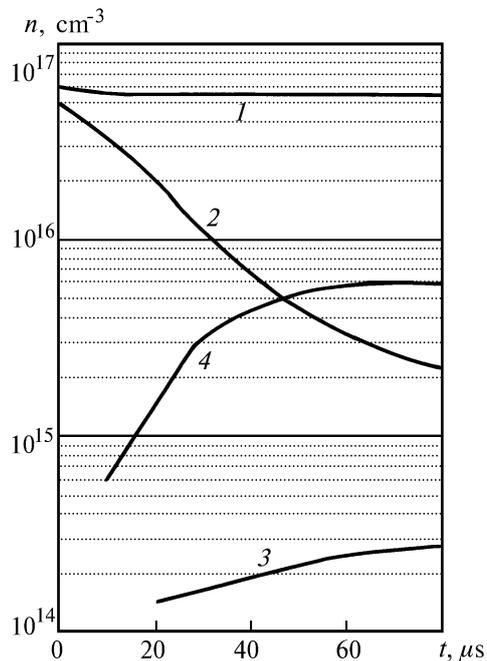
FIG. 3. Temporal behavior of components containing halogen: 1)  $NF_3$ , 2)  $HCl$ , 3)  $F_2$ , and 4)  $Cl_2$ .
