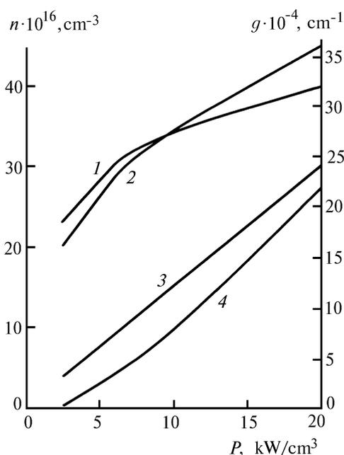
FIG. 2. Optimum Xe concentration (1 and 2) and amplification coefficient of the active medium (3 and 4) as functions of the specific pump power: 1, 3) XeF medium; 2, 4) XeCl medium.
