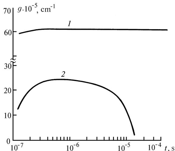
FIG. 1. Temporal behavior of the amplification coefficient for a specific pump power of  $5 \text{ kW}/\text{cm}^3$ : 1) XeF medium, 2) XeCl medium.
