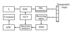
FIG. 2. Schematic of the LFM lidar breadboard construction: laser L, electrooptical converter EOC, and generator of controlling voltage GCV.
