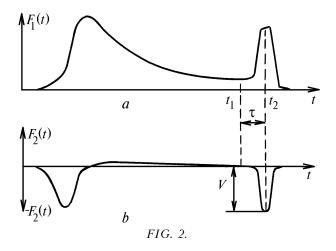
This device was calibrated under controllable conditions using the nephelometric setup<sup>6</sup> placed just near the reflecting mirror. The calibration consisted in determining the proportionality coefficient between the amplitude of the signal V and the value of the lidar ratio at the moment of measurements.
