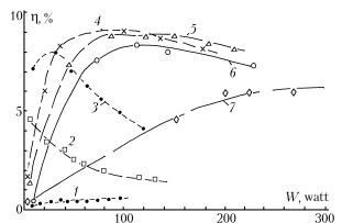
FIG. 1. Efficiency of XeCl\* radiation versus pumping power, Xe:Cl<sub>2</sub> = 3:1 gas mixture at the total pressure < 0.25, 0.25, 0.5, 1, 2, 4, and 6 Torr.
