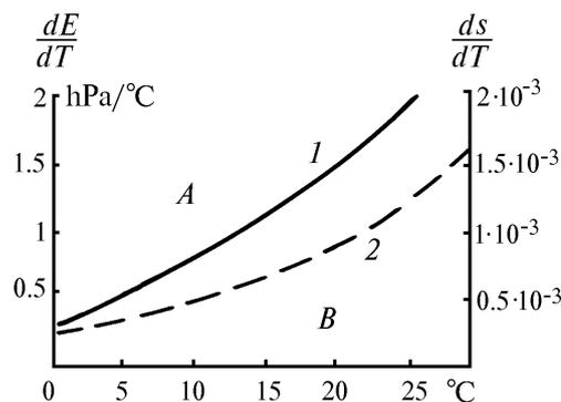
FIG. 2. Cloud track formation behind ship at isobaric mixing of exhaust gases and air as a function of temperature and humidity of the latter as well as the fuel properties. Area A: lanes appear, B: they do not appear;  $dE/dT$  (curve 1) and  $ds/dT$  (curve 2) as functions of temperature.
