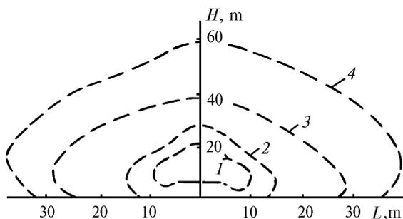
FIG. 1. Shape and size of zones of active turbulent mixing (aerodynamic trail) perpendicular to the ship axis, as obtained from the numerical simulation of the plane ship model at the distance from its bow of 65 (1), 140 (2), 260 (3), and 455 m (4).
